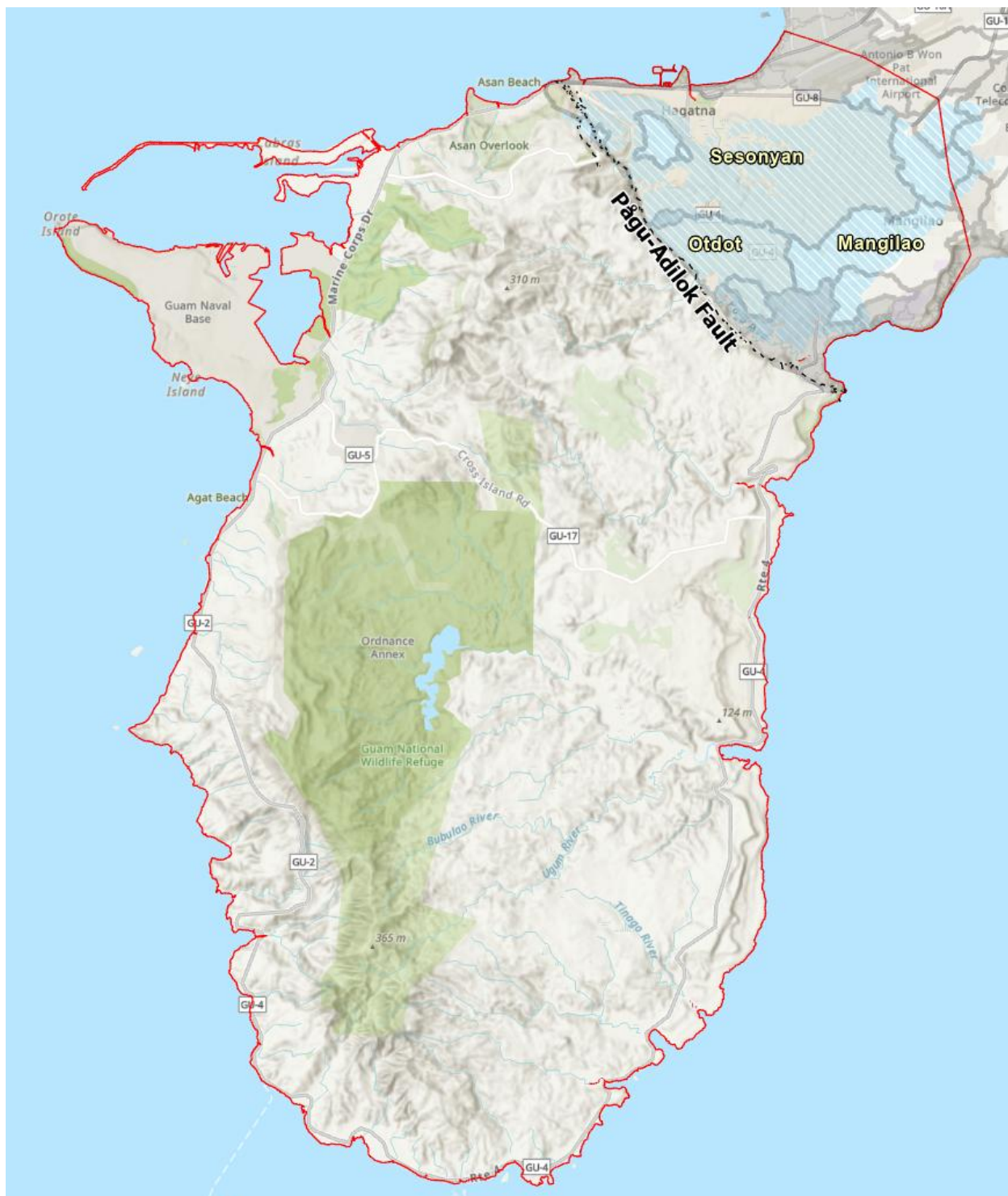
Figure 3.1 Initial domain DEM boundary/area (red line). Above the Pãgu-Adilok Fault are the Argillaceous member (blue-white hash area) and Plateau Basins. The polygon is drawn along the coast and above Sesonyan watershed and Mangilao Plateau Basin.
