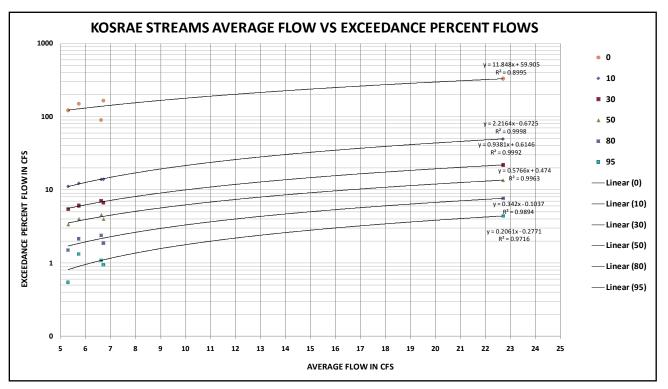
Figure 7. Parametric flow duration curves
