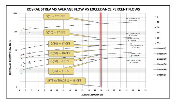
Figure 8. Use of parametric flow duration curves to predict flow duration values at an ungaged site with an average flow of 18 cfs
