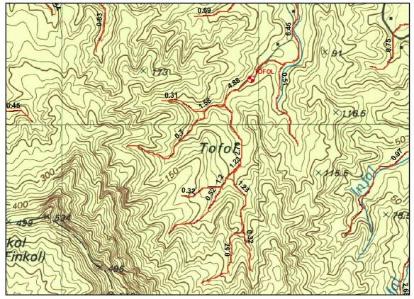
Figure 19. Individual stream reaches on the Toful River showing average annual flow in cfs for the midpoint each reach
