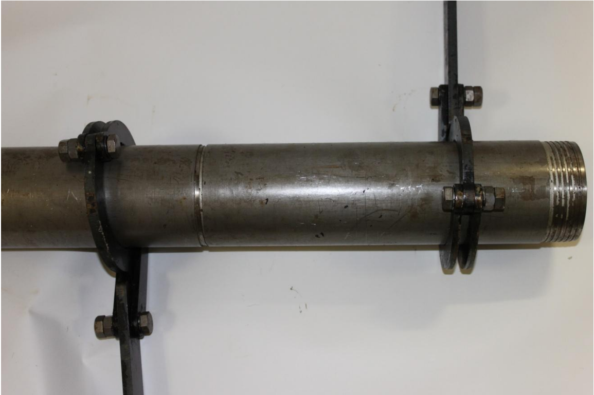
Figure 6. Wrenches to disassemble tubes and bit.
